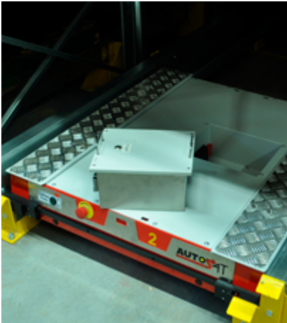
Longlife lithium battery removed for recharging
